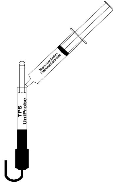
3. Slide the reference sleeve over the plastic stem until the black O ring is 4mm inside the body. Some force may be required. Reference Electrolyte Gel will be expelled from the end of the stem. Rinse with deionised water. Dry the end of the plastic stem with a tissue.
