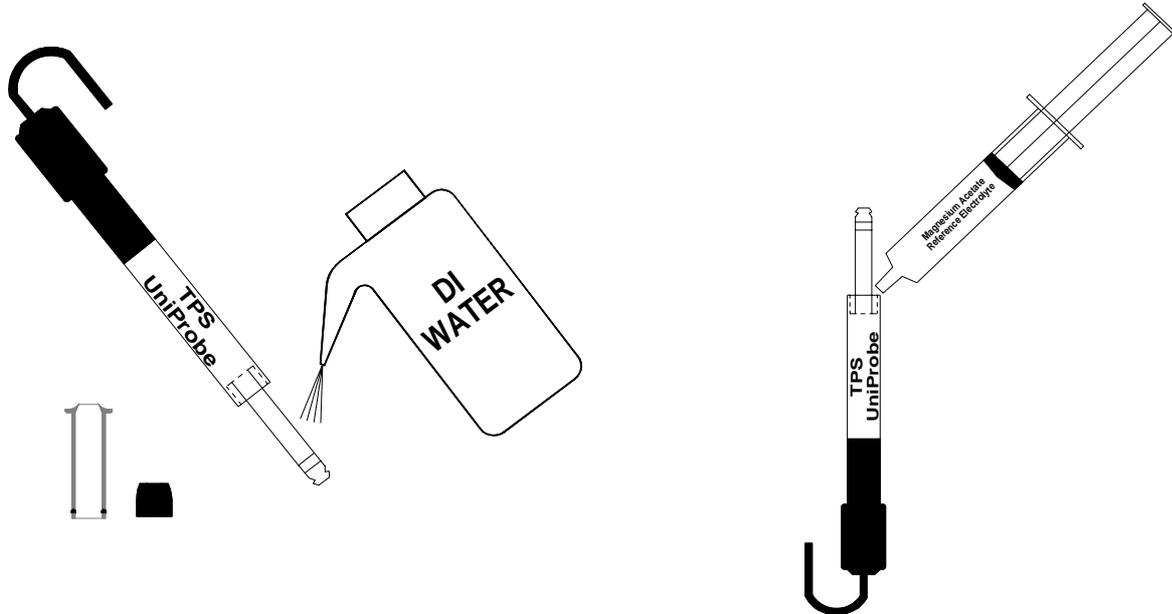
3. Slide the reference sleeve over the plastic stem until the black O ring is 4mm inside the body. Some force may be required. Reference Electrolyte Gel will be expelled from the end of the stem. Rinse with deionised water. Dry the end of the plastic stem with a tissue.
