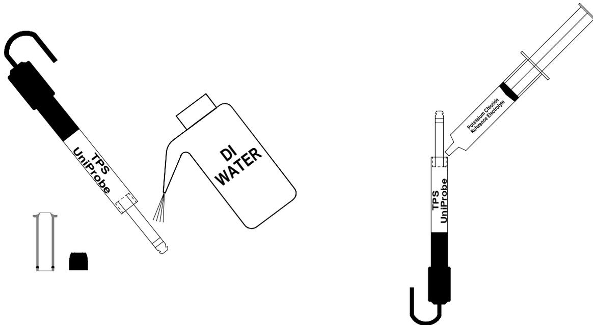
3. Slide the reference sleeve over the plastic stem until the black O ring is 4mm inside the body. Some force may be required. Reference Electrolyte Gel will be expelled from the end of the stem. Rinse with deionised water. Dry the end of the plastic stem with a tissue.
