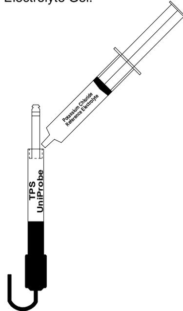
3. Slide the reference sleeve over the plastic stem until the black O ring is 4mm inside the body. Some force may be required. Reference Electrolyte Gel will be expelled from the end of the stem. Rinse with deionised water. Dry the end of the plastic stem with a tissue.
