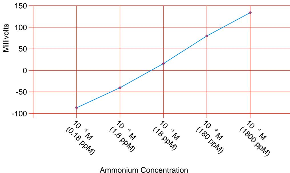
The TPS Ammonium ISE is a potentiometric sensor, meaning that it develops a potential (or voltage) proportional to the concentration of the ion to which it responds. The mathematical equation that describes this relationship is called the Nernst Equation:
