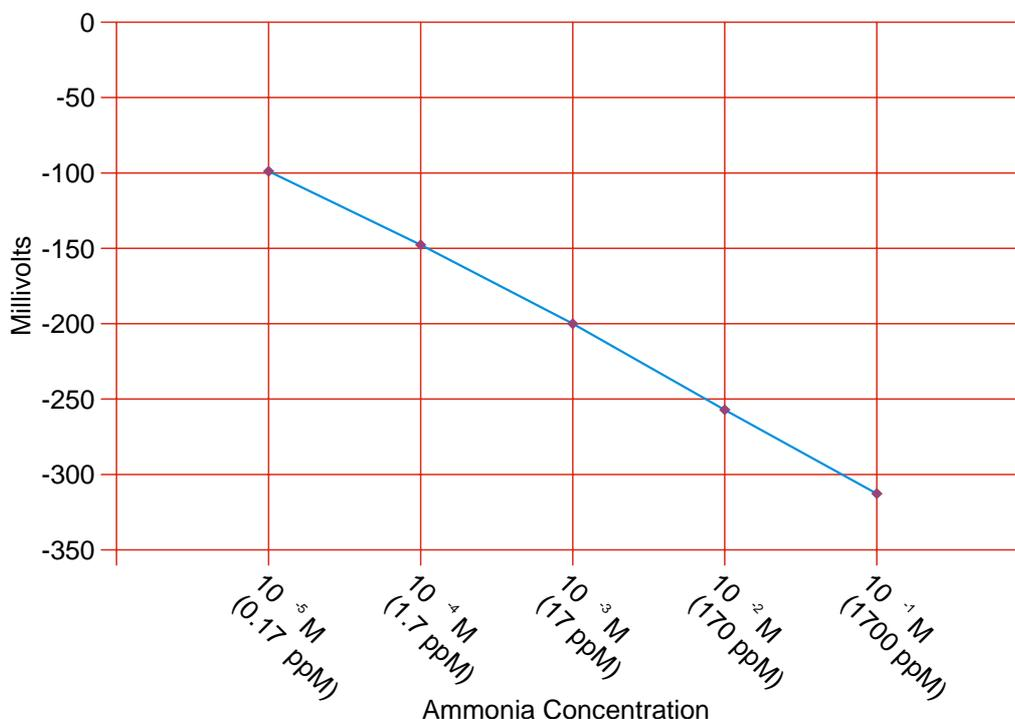
The TPS Ammonia ISE is a potentiometric sensor, meaning that it develops a potential (or voltage) proportional to the concentration of the ion to which it responds. The mathematical equation that describes this relationship is called the Nernst Equation:
