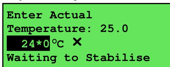
When the Temperature reading has stabilised, the unit will calibrate itself.
