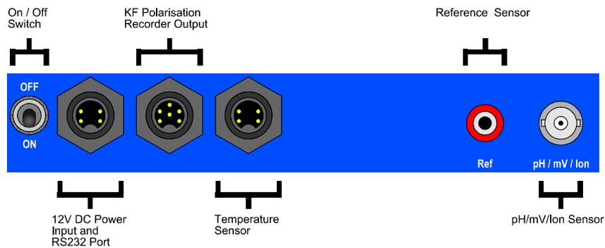
Turn the retaining nut clockwise until it clicks into place when plugging in plastic connectors. This is essential to produce a waterproof seal.
