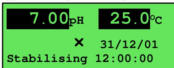
As each parameter becomes stable, the highlighting is removed. If any parameter subsequently becomes unstable, the highlighting is applied again.
