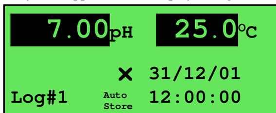
As each parameter becomes stable, the highlighting is removed. If any parameter subsequently becomes unstable, the highlighting is applied again.
