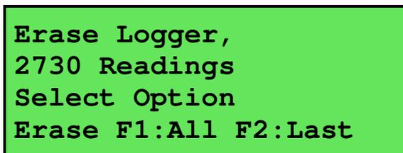
The number of readings stored in the Logger is displayed. See the “2730” in the example above.
