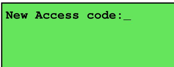
Enter a new code of up to 4 digits using the numeric keypad.
