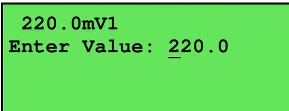
The current mV reading is shown on the top line.
