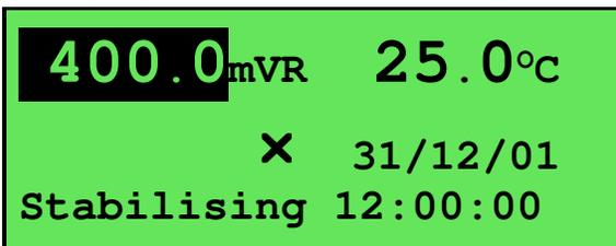
The Relative mV reading will automatically be zeroed once the reading becomes stable.
