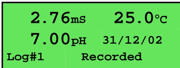
2. Repeat as often as required. The maximum number of readings that can be stored in the Logger is 2340.
