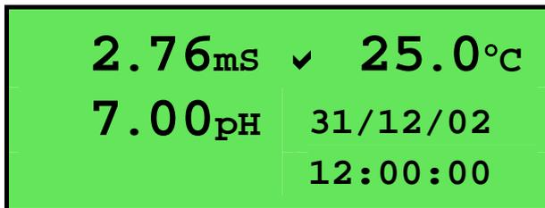
3. To unfreeze the display in order to take the next reading, press  $\text{F5}$  and  $\text{AutoLog}$  again to re-start the ASF automatic datalogging process.
