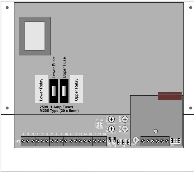
4. Replace the blown fuse with a 250V 1 Amp, M205 type. M205 fuses are 20 x 5 mm.
