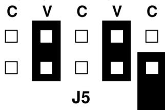
Note that the spare jumper has been fitted to a spare **Current/Voltage Output** jumper pin. This is a safe place to keep it, in case the **proCHEM-DI** needs to be reset to current output in the future.
