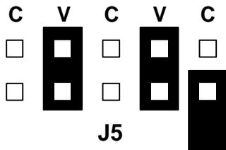
Note that the spare jumper has been fitted to a spare **Current/Voltage Output** jumper pin. This is a safe place to keep it, in case the **proCHEM-D** needs to be reset to current output in the future.
