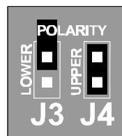
To re-set the action of the Upper and Lower limits to factory defaults, set the J3 and J4 jumpers as shown
