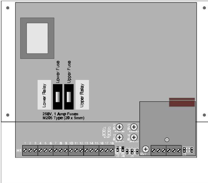
4. Replace the blown fuse with a 250V 1 Amp, M205 type. M205 fuses are 20 x 5 mm.
