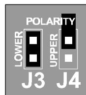
To reverse the action of the Upper Limit, and have two Limits that activate the High and Low LED's and relays when the reading drops **below** the Limits, set the J3 and J4 jumpers as shown.
