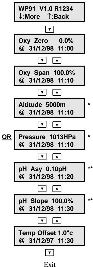
\* Altitude **OR** Pressure are displayed only if either one was switched on at the time of the last calibration.
