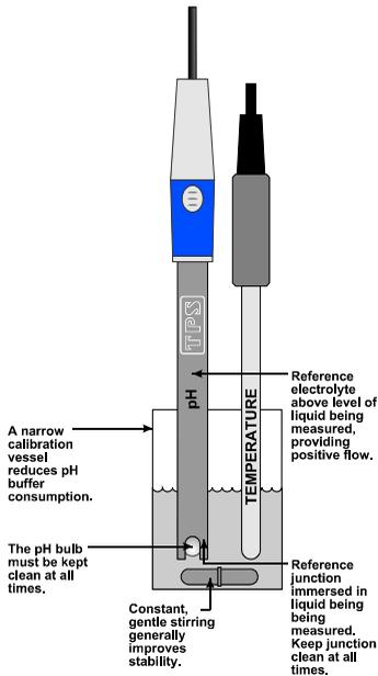
10. When the reading has stabilised, press the **F1** key to calibrate. If a 1 point calibration has been performed, the "\*" will not be removed until a full 2 point calibration has been performed.
