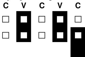
Note that the spare jumper has been fitted to a spare **Current/Voltage Output** jumper pin. This is a safe place to keep it, in case the **miniCHEM-Redox** needs to be reset to current output in the future.
