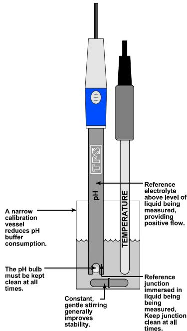
**DO NOT** place the sensors directly into the buffer bottle. Discard the used buffer after use.
