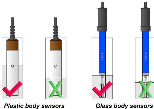
**DO NOT** place the sensor directly into the bottle of standard.
