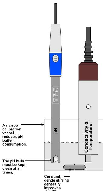
**DO NOT** place the sensors directly into the buffer bottle. Discard the used buffer after use.
