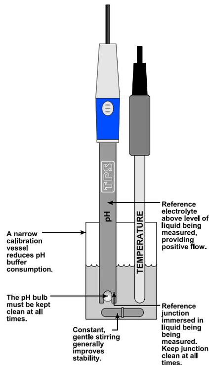
**DO NOT** place the electrodes directly into the buffer bottle.
