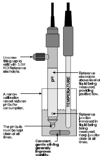
**DO NOT** place the electrodes directly into the buffer bottle.
