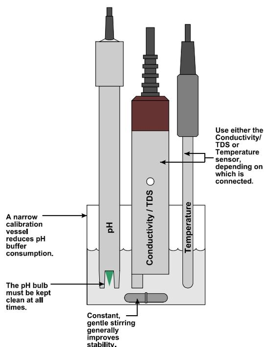
**DO NOT** place the sensors directly into the buffer bottle.
