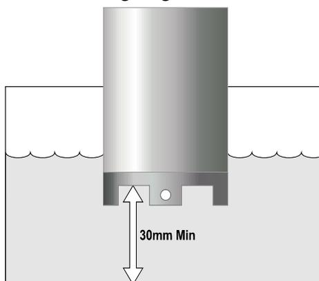
Take care to ensure that there are no bubbles trapped on the underside of the sensor. Bubbles can interfere with Turbidity measurements. Gently stir the sample or the sensor to dislodge any bubbles.
