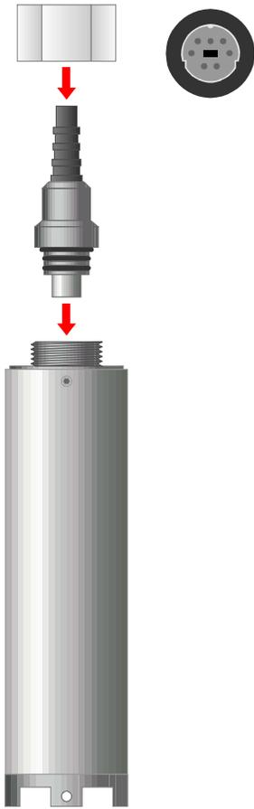
1. Push the cable plug into the socket in the rear of the Turbidity Sensor. Be sure to align the pins of the plug and socket before inserting.
